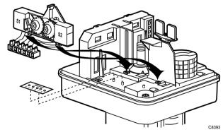
Fig. 2. Installing auxiliary switch assembly.
